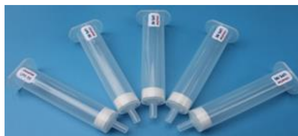
Fig 6.1-3 Photo of ChiralTek UPE90 cartridges (6mL, 90mg)
