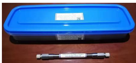
Figure (E). Typical photo of a novel fast ChiralAM-5 column for HPLC to achieve UPLC-like separation
