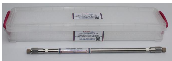
Figure (C). Typical photo of a common analytical ChiralAMCE-5 column
